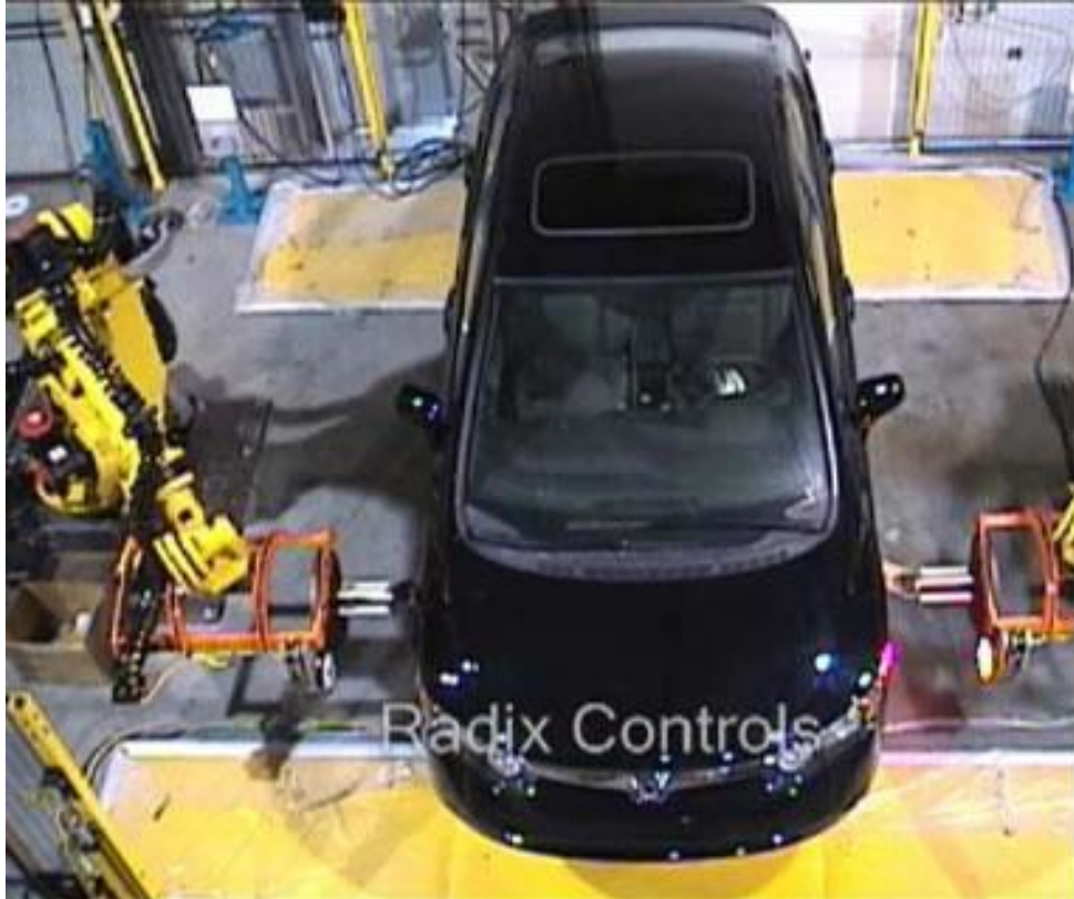
Vision-guided robots position nut runners on wheels
